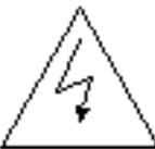
This symbol on or inside the equipment warns of dangerously high voltage.
