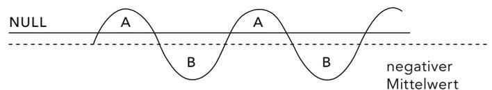
Mean value of an unbalanced AC voltage supply (DC component)
